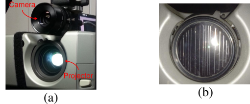
Figure 2. Actual optical system. (a) Setup with a short baseline and (b) coded aperture installed on the projector lens.
